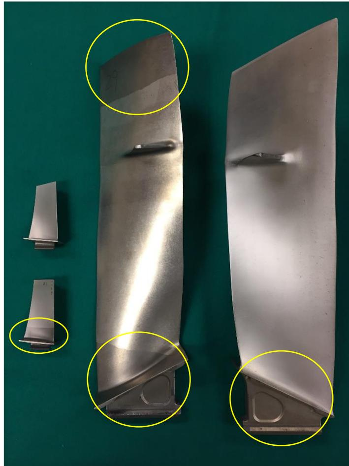
**Figure 3: Laser Ablation cleaned CFM-56 Fan and 1<sup>st</sup> Stage Compressor Blades**
