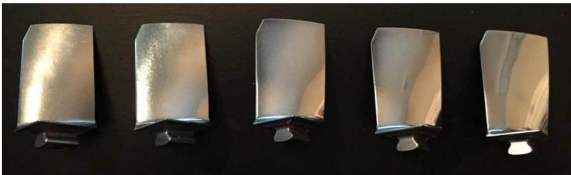
**Figure 7: Comparison of Cleaned and Cleaned / Micro Finished Compressor Airfoils**
