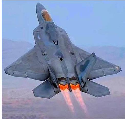
**Figure 8: F-22 Fighter with both P&W F119's in full afterburner**
