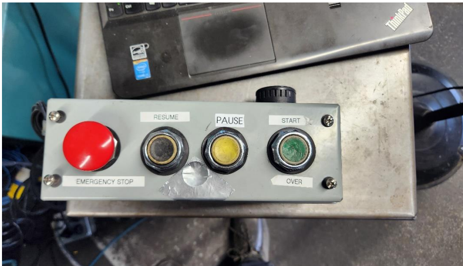
Figure 14: Cobot cell control box with Andon system (speaker alert)
