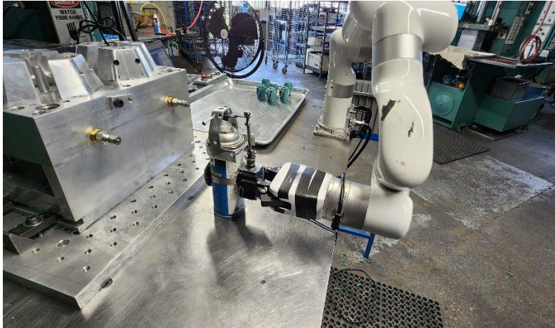
Figure 10: Cobot getting ready to pick-up mould release spray can
