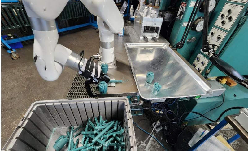
Figure 8: Cobot separating parts from injection runner
