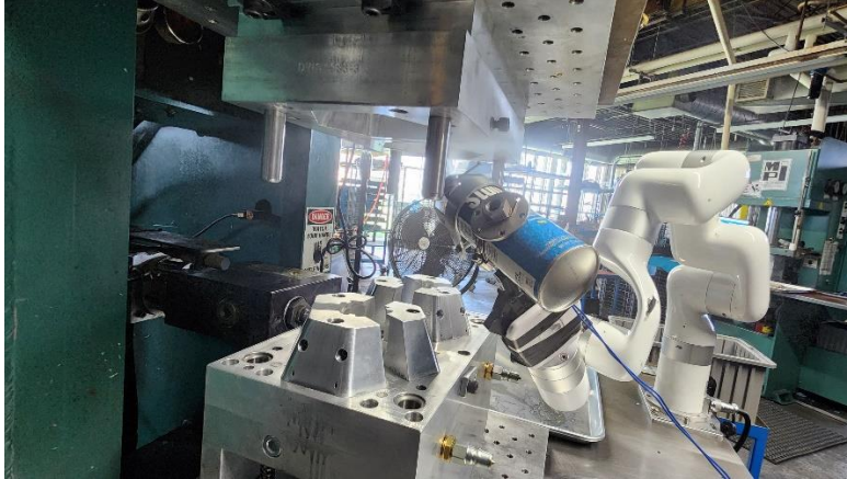
Figure 12: Cobot spraying upper cavity of tool
