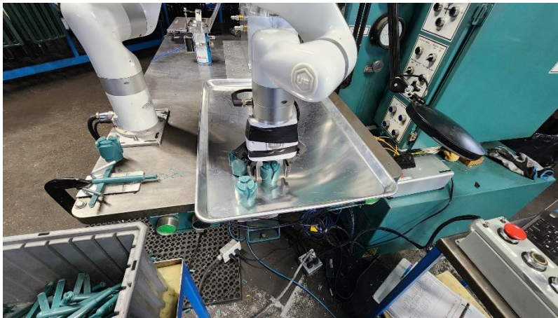
Figure 9: Cobot placing part at the allocated placement point
