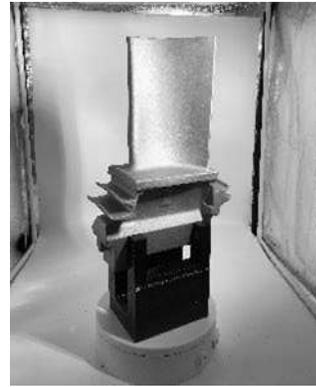
*Figure 13. Completed ABC cast blade, meeting required specifications.*
