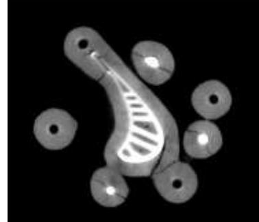
*Figure 8. One slice from a CT image of a conventional blade, with core and shell.*
