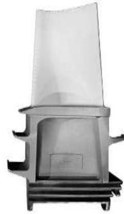
*Figure 1. Finished gas turbine blade manufactured as an investment casting with a ceramic core to form internal cooling channels.*
