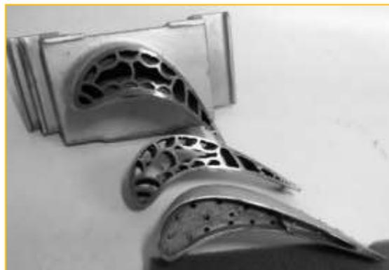
Figure 5. Single crystal blade cast with an ABC core.
