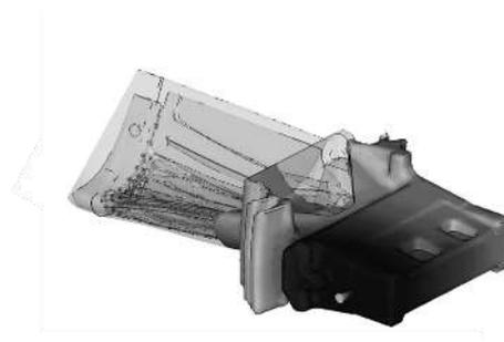
Figure 16. Prediction of wax flow and core stresses during injection.
