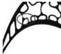
Figure 15. Prediction of location of residual stress during casting
