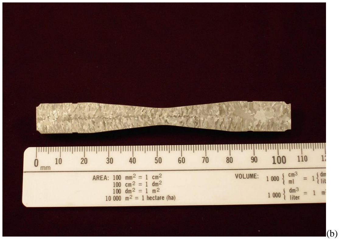
Figure 4. Hourglass shaped test bar of 713 LC. Note the fine-grained structure through the gage section of the test bar in photo (b).
