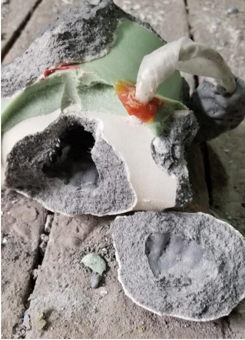
Figures 9-10: Surface of the internal passageway shell and wall thickness showing backup dip quality.
