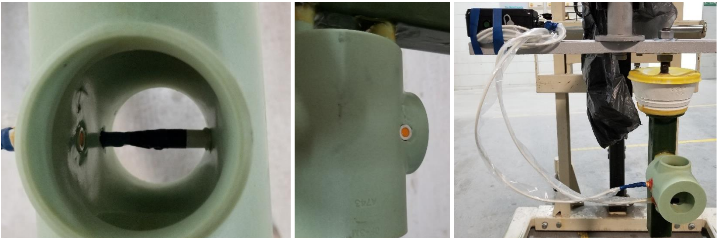
Figure 4-6: Both sensor locations flush with the surface of the part and the staging rig.
