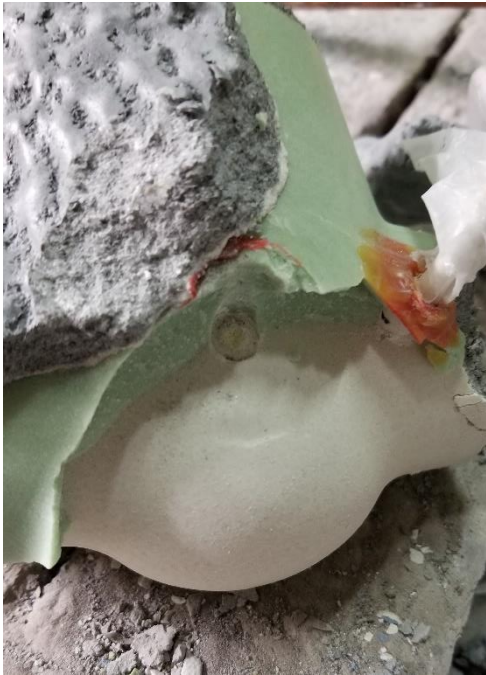
Figures 9-10: Surface of the internal passageway shell and wall thickness showing backup dip quality.
