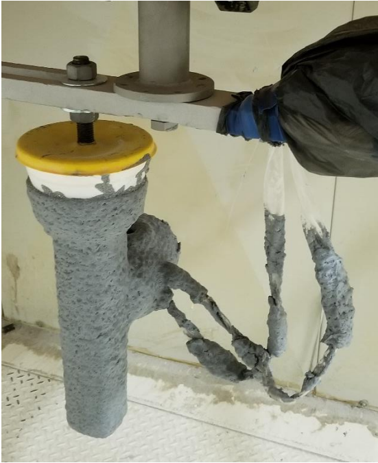
Figures 7-8: Completed part after shelling and the external shell wall.
