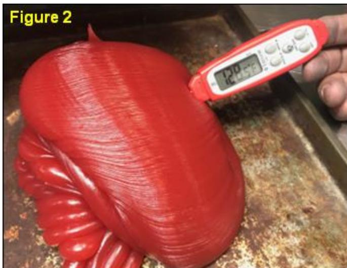
To facilitate comparative injections, Paramelt manufactured a batch of 971 in billet form – the material is usually pelletized. These billets were conditioned in Shellcast’s warming cabinet, sitting at 122°F for at least 48 hours. After conditioning, the test billet was loaded into an Ebbert extruder and used to make test parts.
