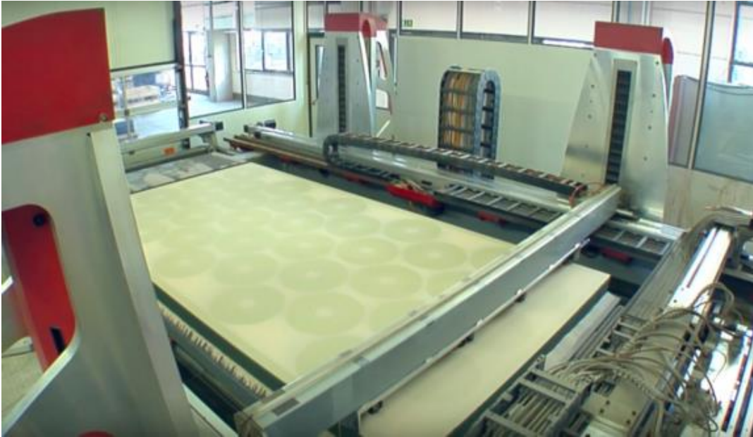
Figure 3 Example of a large bed sand printer used to make both molds and cores. [12]
