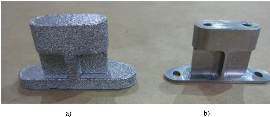
Figure 1: 3D direct metal printed titanium alloy component. a) build geometry and surface finish b) final machined component. [12]
