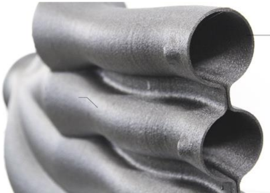
b) typical surface finish of a steel casting made from a printed sand mold [15]
