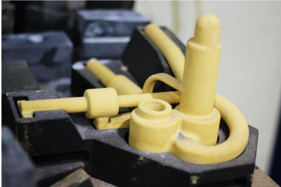
a) example of a complex printed sand core coated with a refractory wash. [13]
