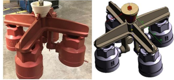
Figure 5. Wax assembly (left) and simulation model (right) of the final setup
