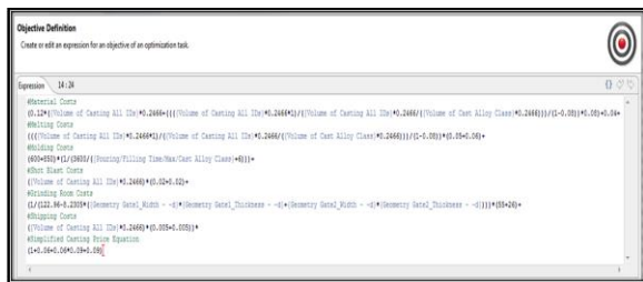
Figure 2. A cost objective has the relevant costing equations derived from the spreadsheet model
