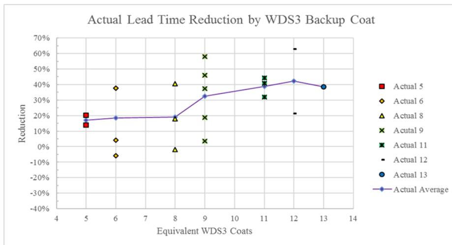
Fig. 8. Observed Lead Time Reduction by Equivalent WDS3 Backup Coats
