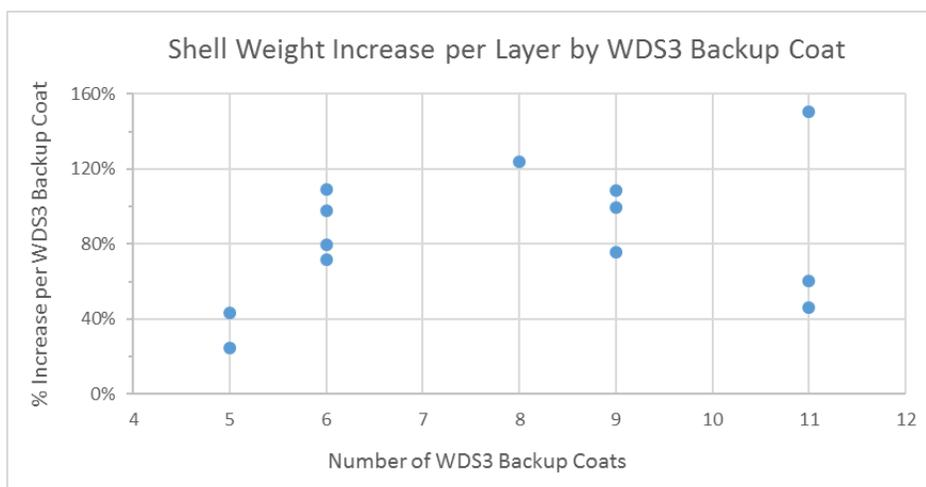
Fig. 6: Weight Increase per Coat
