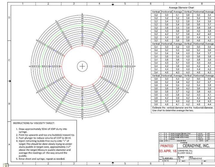
Fig. 3. Target Viscosity Tool.
