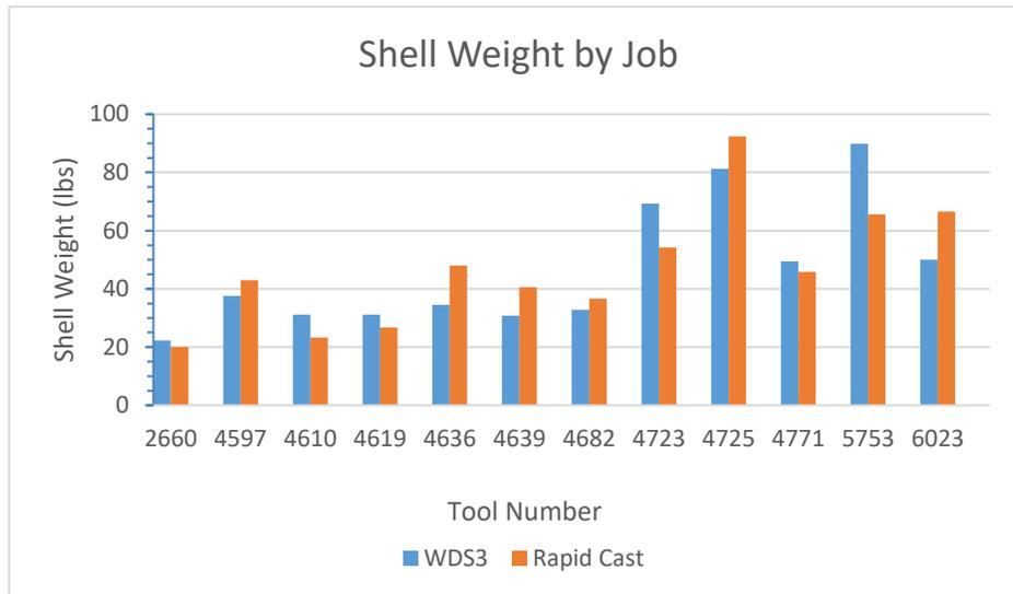
Fig. 5. Shell Weight Comparison (3M™ Fused Silica Advanced Shell System WDS3 vs. 3M™ Fused Silica Rapid Cast System)
